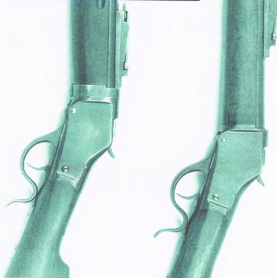
The most noticeable thing about the first generation Winder Musket, right, and the second generation, left, is the position of the rear sights. Placement closer to the eye afforded more accurate aim. The lower Musket is a take-down and, on the whole, more rare than the standard rifle.
